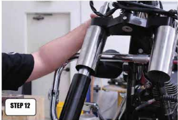
Step 12: Slide fork tubes through fork cans, then through lower and upper triple tree.
